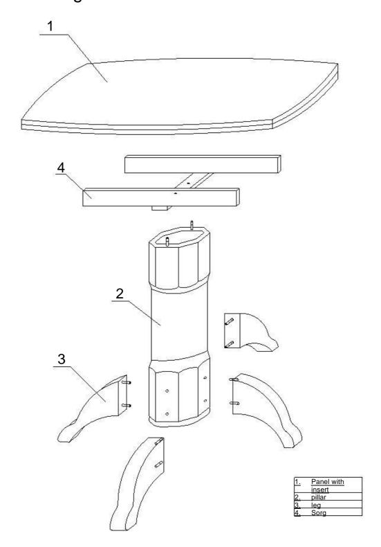
Two persons are needed for montage, the time required for montage is 20min.-Required tool is star screwdriver and wrench no 13.-The legs are mounting first and then the panel of the table .-When mounting the insert , *first release the stoppers that are on the slider* ,open the halves of the table to the end and evenly put/move the insert.
